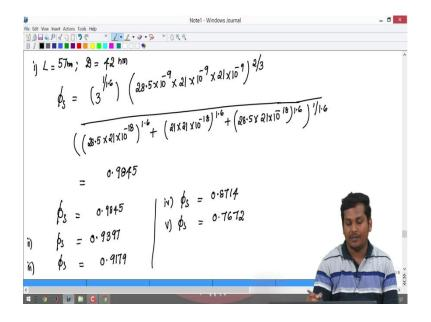
And now we will just substitute those values. So, for the first case we have we were given that the length is 57. And diameter is given as 42 sorry its a nanometers. And we have seen that in the ellipsoid a will be L by 2 and we considered that its symmetric in both the direction. So, b and c are same. So, b will b equal to c equal to D by 2. With that we will calculate the sphericity.
