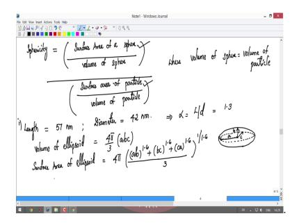
So, first we will see what is sphericity? So, sphericity is defined as surface area of a sphere to volume of sphere, divided by surface area of particle by volume of particle; where volume of sphere equal to volume of particle. So, its actually surface area of sphere by surface area of the particle in which the volume of the sphere and volume of the particle are same.
