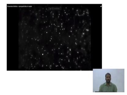
So, this is what has been done is that you know the white dots that you see, these are particles ok. These are something called as a fluorescent particles ok, when people use fluorescent particles the idea is that, if you use a regular optical microscope ok, which works by using the white light, you can see objects up to about a micrometer or larger ok.
