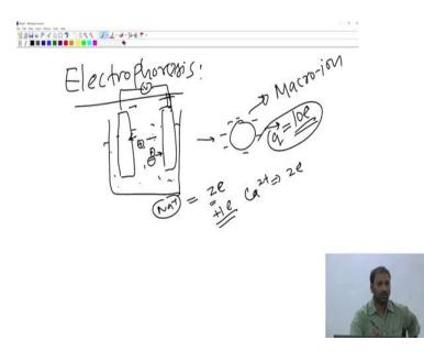
In specific we are going to talk about something called as electrophoresis ok. Now, for electrophoresis so, what you do is. So, all of you know if you have like say, I have a cell say, if I have a cathode for example, and an anode right. Now, if you have ions in solution ok. If, you have like say positively charged ions or negatively charged ions in solution like this is say this is going to be your a fluid right.
