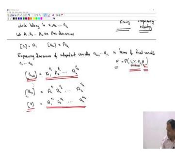
So that means, if I have a k plus one dimensions of a k plus 1 can be written in terms of dimensions of the first k variable let us say A 1 is the dimension of small A 1 which will be raise to some arbitrary power let us say p 1 A 2 to the power p 2 and so on A k to the power p k.
