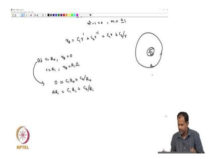
We have an inner cylinder that is rotating with an angular velocity omega. We have an outer cylinder that is static. So, and the inner cylinder has a radius R i the outer cylinder has a radius R o. So, we can say that
