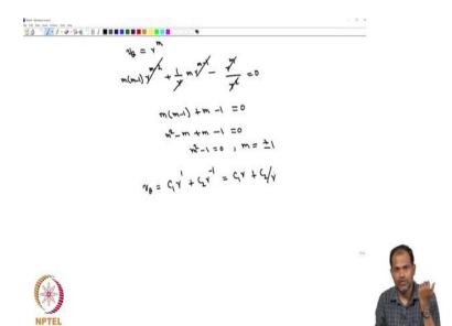
So, these equations are called Euler Cauchy equations and they admit a solution of a power law ok. For example, here the solutions that these equations will be something like r to the power of m. So, that is the kind of solution that we will have. So, we can actually try to find out what that would be. So,
