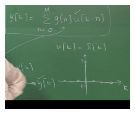
And two, I have cut down also restricted the lower subscript to 0 assuming that the future inputs would not affect the present output. That means, we are assuming causality. We are assuming causal systems. The flow change at a later time, why should I expect that to affect the level now? Under open-loop conditions, that is not true at all, there is no connection between that.
