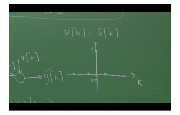
That's why the Gs are called impulse response coefficient. That is, if I punch the system and withdraw, the response that I see is impulse response. The input may last only for one instant, the input lasts only for one instant, but the response lasts for some time. Correct?
