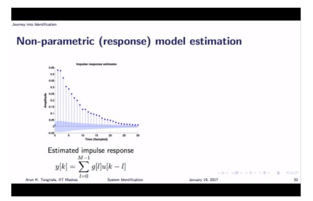
It's essentially estimated impulse response coefficients. The y axis shows the value of the impulse response coefficient and x axis is called the lag or time. There are two things that you should notice. One, let me see if you can quickly pick the first one.
