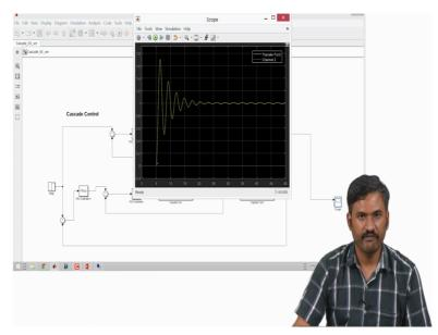
Now I have given the step response at 5 seconds, step change at set point is 5 seconds, as you can see there is sufficiently high oscillations for like 25 seconds, then it settles down into fairly stable response. Now the PID controller is tuned such that we have closed loop transfer function of 1 by 1 1 S + 1.
