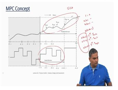
So, just quickly summarising from the last lecture, we talked about Control horizon, which is having a control move plan. So, basically if I am sitting at time T equal to K, if I am making control move plans, since I am still talking about SISO systems here, I have to make
