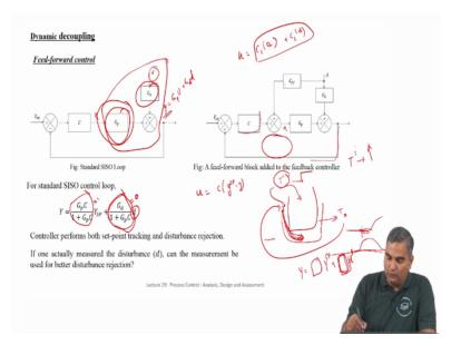
So, let's look at our standard closed loop diagram again here and we have seen this many many times, so just one more time so that we have a context for how this closed loop diagram is going to be modified when we have Feed-forward controller included in the control design. So again standard you have Y compare it with Y set point go through a controller and input Gp and so on.
