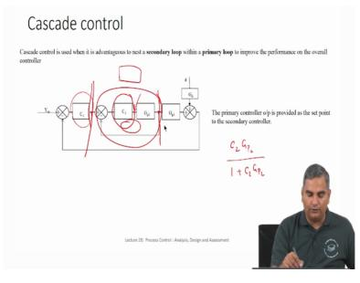
Usually what you do is, the inner loop that is here you first tune and this you tune using a simple p controller because it is fast it is efficient and also remember ultimately there is another controller outside. So if you put a PA controller here you can get rid of offsets and so on. So you do not have to really worry about offsets in the controller inside.
