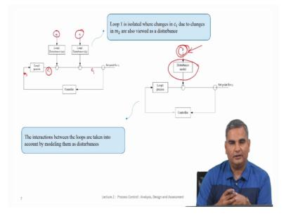
So when we finally look at this what happens is you can simplify this into this blog diagram where you have loop for process one, so which is basically m1 coming in and the effect of m1, c1 because of the effect of m1 here and now I have broken down that pitcher into 2 different pictures. So I'm going to say the effect of m2 which is the other manipulated variable you might want to think of that as a disturbance that changes the value of the control variable C1.
