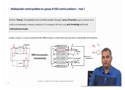
So let's kind of think about how that large problem is broken down into smaller problems, the reason why am showing this year is to give you an idea of how for realistic, for real industrial problems we start from an overall concept of control which is inherently multivariable and then we break that down into single input single output controllers and think about single input single output controllers for the next 15 to 20 lectures.
