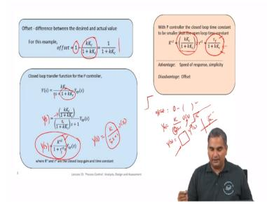
So the offset you might define as the difference between the desired and actual value so for that example that we had offset because I give step of one the ultimate desired value of one but the value that output takes T tend to infinity Y of T is KKC by one plus KKC, so this if you do some
