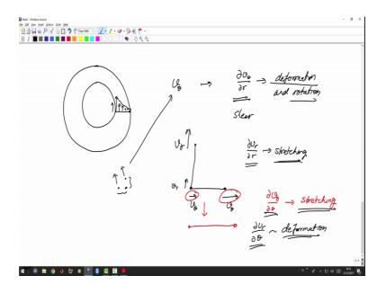
We have an inner cylinder which rotates with certain velocity and then the outer cylinder which is kept fixed and because of this the flow profile is again where the inner cylinder keeps on moving and therefore, the velocity would be something like this. So, the velocity decreases and goes to 0 at the top edge. So, again if we keep some, so in this case, we only have v theta and again del v theta by del r will indicate about deformation
