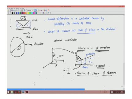
So, cone in plate as we will see later on will be a device in which case; we will have a cone which is rotated at a given controlled speed it could be also oscillated and then we have a plate. So, we have a cone and we have a plate and the fluid of interest is actually taken in the gap. So, this is where we take the fluid of interest which could be let us say ink, it could be paint, it could be polymer melt, it could be a paste, whatever is the
