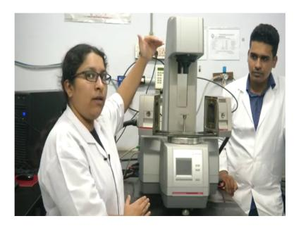
The rheometer has the head, in which you have the main components that help in the functioning of the rheometer. So, the rheometer has an encoder a motor and a air bearing. The purpose of an encoder is to monitor the extent of deformation that is being that is a rheometer that is what the rheometer has to do. what the motor does is, it basically converts the mechanical energy to the electrical energy so that the equipment can understand.
