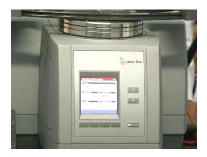
So, once we switch on the rheometer, we look we have to establish communication with the equipment communication between equipment and the software ok. So, once you open the software, the we need to initialize so as to establish the communication.
