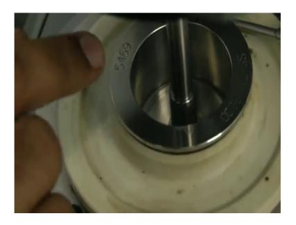
So now, we will see inside the rheometric geometry where we can see that the mixture is de mixed state and we will see a turbid solution towards a side in annular region of the concentric cylinders. So, first we have to filter the samples in a concentric cylinders in a geometry, and now it is a de mixed it.
