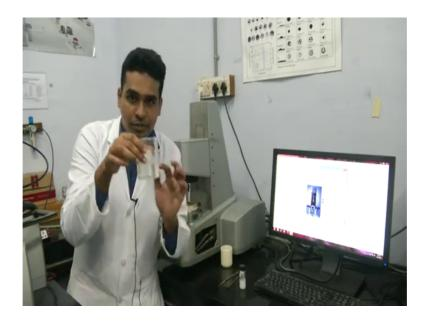
So, what you will observe is as you increase temperature, and we go from a clear solution to turbid solution, you will see increase in moduli and the viscosity. So, oscillatory shear is one way of characterizing this transition from what you say clear state to do a high viscosity state in this case ok.
