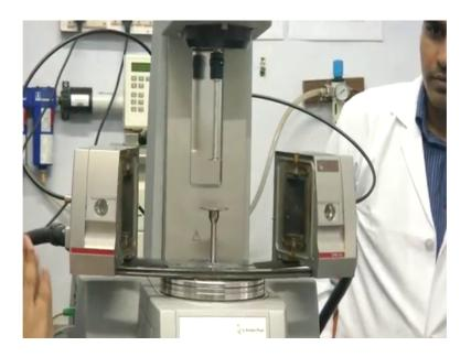
So, for example, let us consider a measuring system that we generally talk about in class. So, this is the cone and plate system with a very small cone angle.
