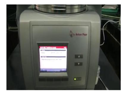
Now, it is at a measuring position and we can start the test now, and we see the variation of the viscosity and the stress shear ok.
