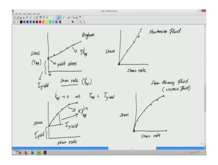
So, in this type of an experiment what we are trying to do is the following that, we subject the material to different strain rates and we are measuring stress. So, what would happen is basically if we choose a one particular strain rate, we may get one value of stress and then if we continue these measurements we may let us say collect these data points. And if we go to lower and lower strains basically what we have is stress
