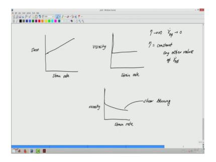
So, where we have stress versus strain rate since we saw that the overall behavior is like this. So, in this region viscosity is constant. So, if I were to plot viscosity as a function of strain rate, what I would see is viscosity is constant and then at strain rate going to 0 there is a finite stress value. So, stress divided by strain rate which is 0 the viscosity is infinite.
