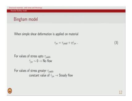
A simpler model which was proposed by Bingham and in fact, now this is an idea which is about 100 years old. So, Bingham proposed that stress in the material is related to yield stress, and the overall stress beyond an yield point is basically like a Newtonian fluid. So, we have also seen example of this.
