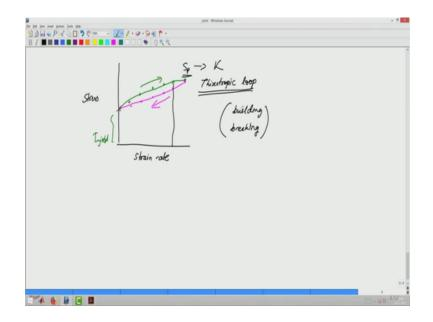
And so, what we saw is if you are measuring let us say stress versus strain rate, in that case what we saw was the measurements were done such that we saw that at low strain there was a finite yield stress value, and even if you extrapolate there is a finite yield stress value. Now once the strain rate is increased and now the same sample if we start measuring the material response.
