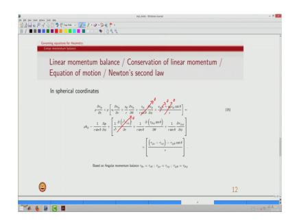
We should be very careful in terms of using. Now this term is actually the centrifugal acceleration that we are familiar with rho v theta square by r. So, this is actually a component r direction component, and in r direction we have of course, velocity in r direction and the stresses which are in also r direction though they may be on different surfaces, and we can see that in this balance we also have ah term which is due to the flow in theta direction.
