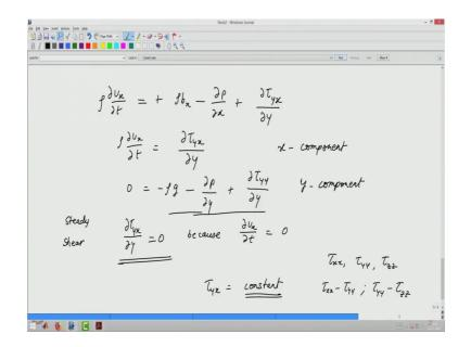
So, let us write it down in the governing equation for this parallel plate flow is del v x by del t rho is equal to plus rho b x minus the gradient in x direction plus what we know is we do not have any information. So, therefore, we only know del tau x y by del y.
