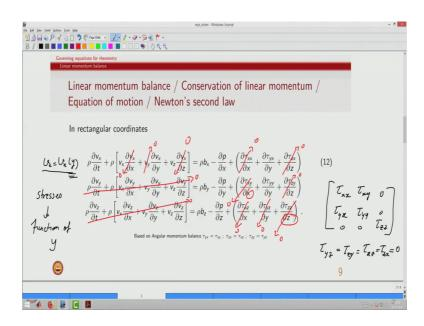
So, now this is the linear momentum balance for in rectangular coordinate, we remember that angular momentum balance ah is ensures that the stress tensor is symmetric. So, that tau y x is same as tau x y tau z x is same as tau x z and tau z y is same as tau y z, and given that the linear momentum balance is a vectorial equation we have 3 components the first component is the x component.
