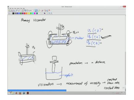
And if you look at Mooney viscometers geometry it is a shaft with rotating member which is a disc, and then in that there is a chamber. So, there is a chamber in which the fluid is kept. So, the in rubber in this case will be kept in this gap, and then the shaft is rotated ok.
