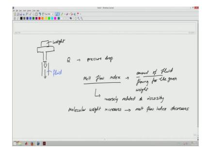
And through which the material has to flow we know that the amount of material will depend on the pressure drop, and this is true whether it is a Newtonian fluid or a non Newtonian fluid. So, in case of the melt flow index what is done is there is device let us say a piston kind of an arrangement which is kept which will push the fluid. So, the fluid is kept in the capillary, and then it is pressed using some weight here. So, there is a weight placed.
