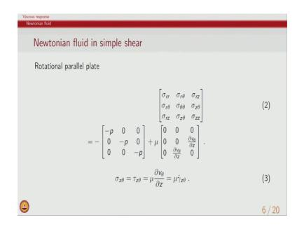
And the top plate is being rotated and the fluid is kept in between and, since we have this simple shear flow we have velocity in theta direction and it is only a function of z. So, therefore, the only component of velocity gradient which will be most relevant in this case is del v is theta by del z and that is what we have stated here.
