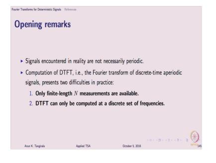
One is that the signals encountered in reality are first of all finite in length and they are not necessarily periodic of course, right that is the first issue; I have only finite length measurements and secondly I have a computation issue, I can only compute or a grid of frequencies. So, these are the two issues that we have, so keep the d t; f t in mind and ask this two questions.
