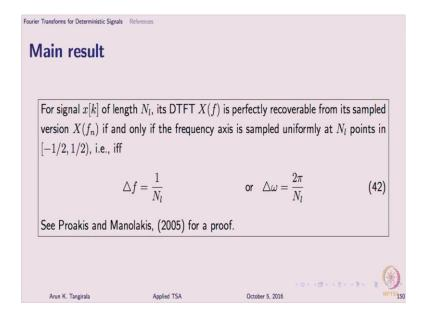
When delta f n is 1 over n l; that means, if I have 1000 points that is 1000 observations of a signal, the frequency grid is of spacing 0.001 and what this also tells me is that I will compute by the way I can notice from the property of by the way is f n let me first tell you what is the f n; f n is now n by m, I will throw away the subscript now.
