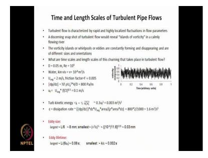
We estimated that for flow through a pipe at a Reynolds number of 10 to the power 5 that is 1 lakh. We estimated the size of eddies and the lifetime of eddies which is of the order of fractions of millimeter and a few milliseconds is the time fluctuations associated with this eddies.
