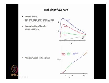
For example, this is a typical variation of u prime square bar, and v prime square bar, w prime square bar, and u prime v prime bar in pipe flow and these are varying we will see more about this with respect to space and so these are not zero.
