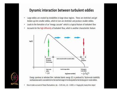
We also made the point that eddies of different sizes are there, we have very largest eddies which are created by instabilities in regions of high shear; and through the action of hydrodynamic forces, as a result of a fluid motion, these eddies get broken up into smaller and smaller eddies. And the smallest size that can be sustained is the Kolmogorov eddy size which we said was of the order of 0.1, 02 millimeters.
