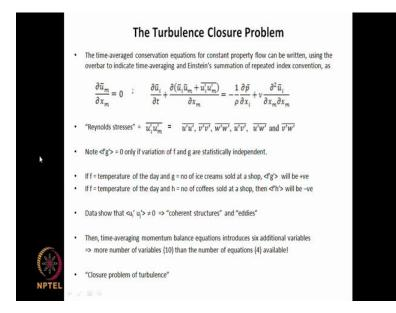
So, if these are not zero, and these are remaining in the equations so that means that this set of four equations that is one continuity equation, three momentum equations, we have four equations. And the feature 10 variables you have the three velocity components that is u bar, v bar, w bar, we have p bar the pressure the time average pressure and in addition to that you have these six components six terms which are known as Reynolds stresses.
