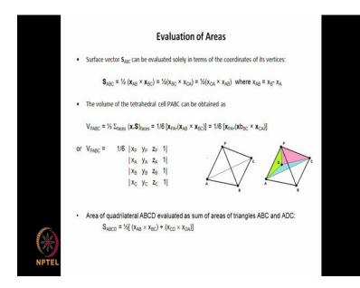
So, evaluation of areas surface area of vector S ABC can be evaluated solely in terms of the coordinates of its vertices. So, S ABC is given as half of the cross product of x AB and x BC, it is also the same as x BC and x CA. So, you can see that and x BC or x AB is x B minus x A, where x is the vector consisting of the three coordinates x, y, z coordinates of point B and x, y, z coordinates of point A.
