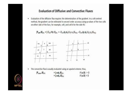
So, there is another aspect to fluxes, fluxes have the diffusive component and the convective component. Diffusive component will introduce the gradient of flux; convective components will involve the value or the flux itself, the absolute value of the flux and not the gradient. Now how do we do this? The diffusive flux requires the determination of the gradient in a cell centered method like this; the gradient is evaluated using the cell value here and the cell value here.
