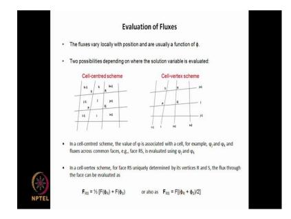
Now, flux is F dot S, we have seen how the surface area vector can be evaluated from the coordinate positions of the vertices. Now how can we evaluate the fluxes and fluxes very locally with position and they are usually function of phi.
