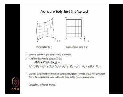
We saw in the previous class that if you were to use a body fitted grid then we would work in the computational plane where you have uniform grid spacing in both psi and eta directions. This psi and eta directions are such that lines of constant eta example this line will be a curvilinear segment here; and some of these boundaries here are such that they fit into the boundaries that are present in the physical plane.
