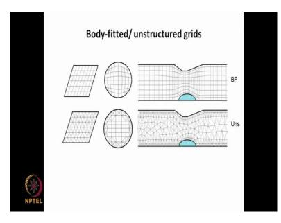
We are looking at the two possible ways of dealing with this one is the body fitted grid the other is unstructured grid.
