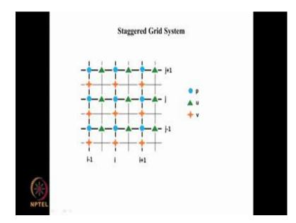
And the way that that is proposed quite early on in the mid sixties itself was to use a staggered grid system. We know that we are solving different variables using different equations. We have seen that the x-momentum equation is used for getting the u variation, and we solve the y-momentum equation for v, and we solve the continuity equation for density or pressure like that.
