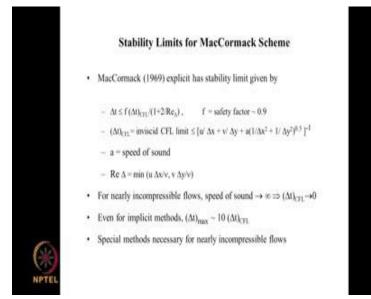
Now, because this is an explicit method it has stability limits potentially stability limits and when you have these coupled equations and when you have non-linear equations all these complications; when these complication arise it is not possible to get an exact analytical expression for stability and so the Mac-Cormack have estimated the stability and express this time step delta t that can be taken in using the factor of safety f. So, this is delta t must be less than f times delta t CFL.
