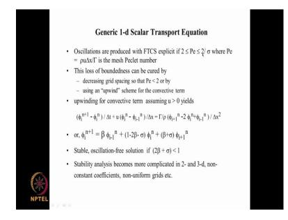
The solution itself can give us to oscillatory solution, oscillations and these oscillations are in the special direction not with the respect to temporal thing, under certain conditions that is if you define a Peclet number and mesh Peclet number as rho u delta x divide by sigma where sigma is diffusivity and u is obviously the velocity and dou is the density.
