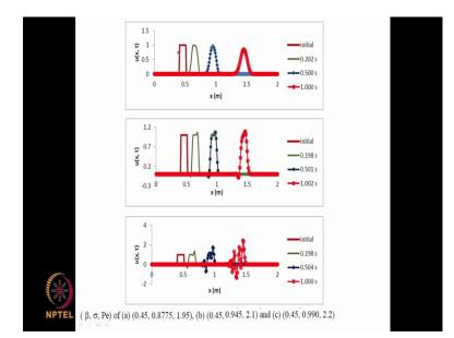
So, that is what we can see here these are an initial square pulse lying between 0.4 and 0.5 at time equal to 0 with a value of 1 here and 0 otherwise, that is the initial condition. We are going to look at how this pulse is transmitted in the x direction at the velocity u while it is also diffusing. So, the evaluation of this square pulse is subject to this equation here. So, it will both be convicted in the positive x direction and is also diffusing with a diffusivity of this.
