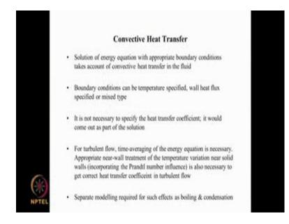
And what we need to do is that we (Refer Time: 08: 26) equations and we identify the domain, and we specify the boundary conditions so that is all we need to do, we do not have to do anything special for convective heat transfer. So, the boundary conditions what do we want here we want boundary conditions can be temperature specified, wall heat flux specified or both can be specified.
