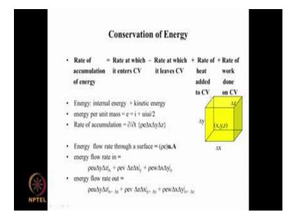
And the statement that we make about the conservation of energy is that the rate of accumulation of energy possessed by the fluid, within this control volume is equal to rate
