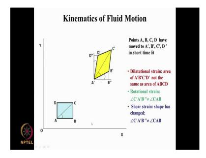
So, this is what we will see in the kinematics of fluid motion and we have put the essentially the same thing here and some color. We have x y coordinate systems and you have points A, B, C, D with some defined diagonal angle here and after short time A has gone to A prime, B has gone to B prime here and C has gone to C prime and D has gone to D prime.
