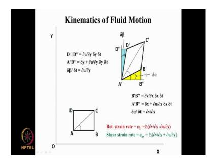
So, that is what we have saying here. Now we need to here we have identified angles delta alpha and delta beta and what is delta alpha delta alpha is the new angle that the side A B makes with a horizontal here it is zero and here it is delta alpha. That is because B has moved up with respect to a relative to A both A has moved up to A prime and B has
