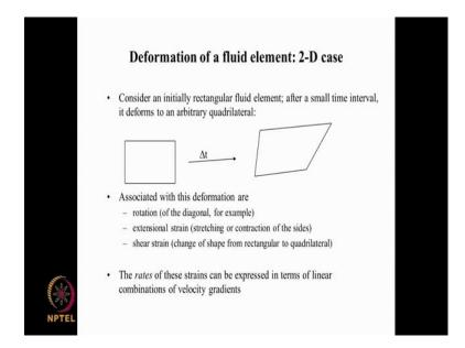
For a fluid element, by looking at the deformation of the fluid element and deformation fluid elements and all these things is in general 3-D, but in order capture the essence of it
