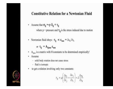
On the way, this we can go back to our original formulation and we can very briefly touch upon how we can derive this Navier-Stokes equation. So, we have the stresses sigma i j and we first decompose this into two components pressure, which is a known property of fluids and we know the pressure is compressive. So, we put it as minus p delta i j we also know that pressure is normal.
