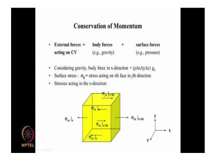
So, this particular cube this box has six faces positive right face, left face, bottom face, top face, back faces and front face. So, the stress acting in the x-direction on each of
