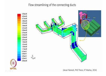
So, if you look at what can be done is we are looking at just this ducting here which is taking the combined flow after it goes to the true air free heaters and then, it is spread into this e s ps. So, we are looking at how to make the fluid distribution even at the four exceed points here, at the four exceed point despite the facts that is coming through bends here, bend here and bend here angled in and all these things.
