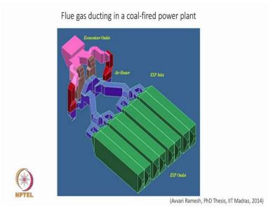
This is a typically example of how fluid flow occurs in many process industry applications. What we have here is part of the gas ducting. Above this is a large duct which carries hot air hot fluid gas from the furnace and it enters here. At the time it enters here, it is still at some 500 degree centigrade. So, there is a lot of thermal content within this and this needs to be exploited, so that the overall efficiency of the thermal power plant is high.
