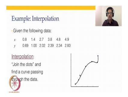
Now what is interpolation? Interpolation, is kind of joining the dots which basically mean that we want to find a curve that passes through all the data points. The reason why we would use interpolation is for example fill in the missing data. So, let us say this is the particular set of data, and we want something at 2.0. See there is no data available at x = 2.0. So, in that particular case, we are going to use interpolation.
