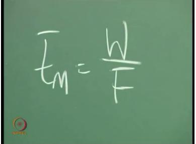
And, again as usual I am giving you. If I give you t bar m that is a for existing reactor. Where you know already t bar m is nothing but W by F. Where W is the holdup of solids inside the reactor and F is mass flow rate of the solids, okay. Normally, it is in homogeneous system it is volume by volumetric flow rate but here we go for mass. Yeah, weight by mass flow rate of solids, okay, good.
