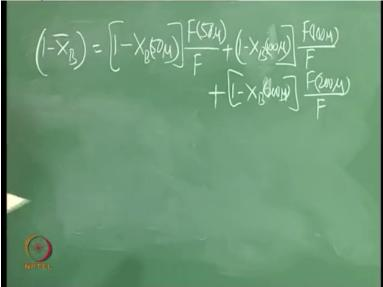
So, I will write the general expression. I think, I will go that side 1 minus X bar B equal to - we have one minus XB for 50 micron particles into F of 50 micron particles by F plus 100 micron particles again F of 100 microns by F. I think I have to write here only. So, 1 minus XB of 200 micron particles. Yeah, that is the equation, okay.
