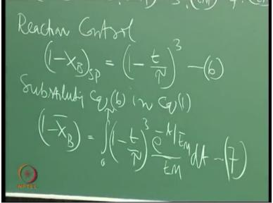
So, now, equation 6 is again substituted in equation 1. Substituting equation 6 in 1, let me write the equation 1 minus X bar B equal to 0 to Tau, for this one it is 1 minus t by Tau whole cube t bar m by t bar m dt. So, this is equation 7, good.
