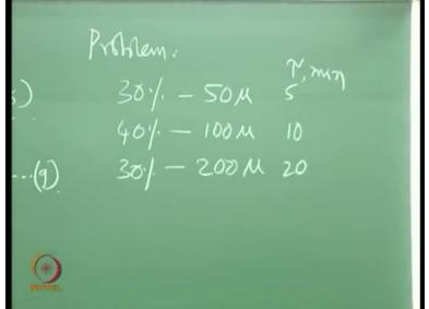
That means, here, I have Tau minutes 5, 10, 20 for three size of particles, okay. Find the conversion of solids for a residence time of 8 minutes in the reactor - very nice problem! So t bar p is 8 minutes, yeah, Tau are given, Tau for 50, Tau for 100, Tau for 200.
