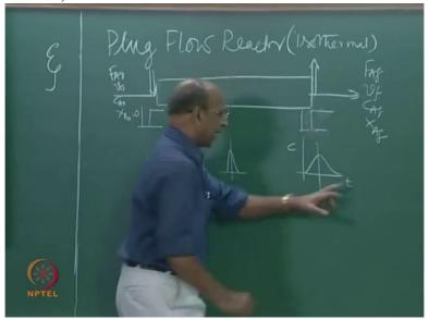
At this end if I see, so that means the, the molecules which are here, the front portion when it is moving, those things will come first and later at the center and later at the back.
