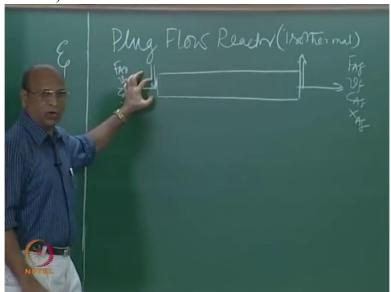
Then I will also have another stream of red fluid, red Ok, so then at time t equal to zero, I will switch off this, there is valve here, and there is another valve connected, the moment I switch off this valve, another valve will open exactly same flow, same flow, no disturbances, not allowed.
