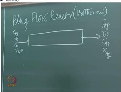
you know water is continuously flowing. By somehow, it is only imagined experiment, by some imagination, I will just assume that, Ok, disk suddenly entered the cross-section entirely fitting there, exactly fitting there. It is uniform cross-section. Even though I have written slightly bulked here, bulk there, I think you know it is exactly same cross-section. How does that move? Moves as?
