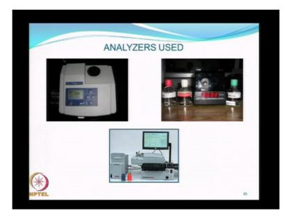
Some of the analyses that are used for testing particle compositions and sizes and counts are shown here. The left inside top picture shows a turbidity meter, may recall that we discuss this in the context of measuring particle concentration since suspensions. Turbidity is a measure of the total scattering intensity of particles in suspension. So it can be used as a qualitative measure of particle size as well as particle concentration in liquids.
