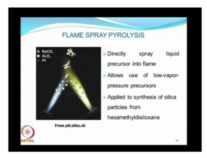
Flame spray pyrolysis is a combination of 2 methods that we have discussed earlier flame pyrolysis and spray pyrolysis. Here the liquid is sprayed directly into the flame so the liquid precursors are injected into the flame. The advantage of this method is that you can use low vapor pressure precursor because the combustion process will supply sufficient heat to vaporise even low pressure precursor materials and this is applied to synthesis of silica particles.
