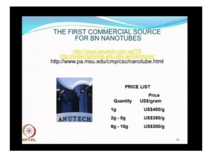
In fact a high-energy ball milling combined with thermal annealing was the first commercial process to be used for the production of boron nitride nano tubes and cost wise actually this is very competitive with bottom-up approaches. You can see some prices listed here for grams of material, in comparison if you are trying to make the same materials using a bottom-up process it would cost you at least 3 to 4 times as much.
