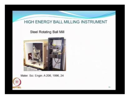
However more recently there have been advances in ball milling technology in particular the high-energy ball mill which is an improvement over the conventional ball mill in the sense that it is a more controlled operating environment. Say can actually control the temperature inside the milling chamber, you can control the pressure, you can even control the chemistry of the ball milling chamber in order to produce the product that you need.
