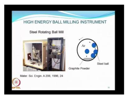
This is again a schematic of how a high-energy ball mill might look, essentially the mechanism remains the same you are still taking material to be size reduced putting it in a chamber and allowing the grinding media to impact on the material with some force which causes the size reduction to happen. However in this example you can see that the inside of the chamber is filled with argon and inert material to prevent oxidation.
