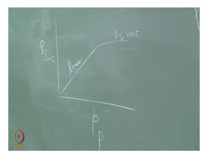
Another example as we are trying to incorporate phosphorus into silicon people have done studies of how the partial pressure of phosphorus influences the phosphorus incorporated into the silicon and what you find is you get a linear relationship for a while but then the slope drops and it becomes more of a square root relationship. Now this is actually difficult to predict because normally you would expect that this should be essentially a linear dependence.
