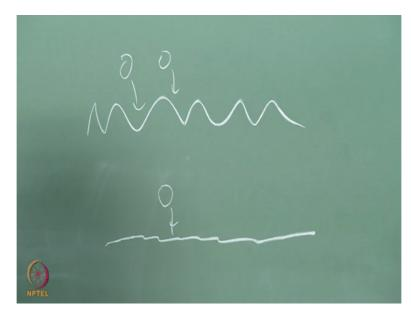
For example if you have a glass surface that looks like this and let say that by putting in some additives and flowing it at high-temperature you have been able to make it look much smoother on a microscopic scale, when an arriving molecule sees this surface versus this surface the effect of surface roughness on capture efficiency or sticking probability is different depending on the scale of the roughness that is present on the surface.
