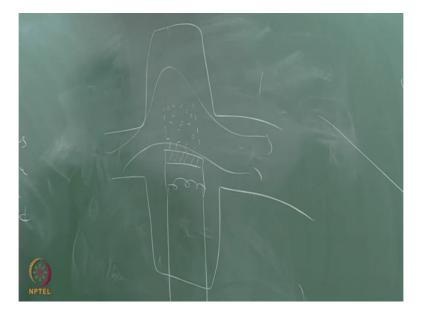
So for example in a CVD reactor, let's say you are using a conventional flat plate type of CVD reactor and you have your wafer here and the gas flow, you know, is like this. If you want to use this as an aerosol CVD reactor, the aerosols should as far as possible be formed in a region that is directly above the substrate, so that they will naturally just by gravitational sedimentation other body force effects by inertial effects drop-down on the substrate and deposit there.
