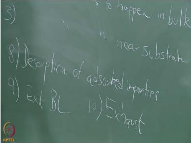
So all the unreacted gases, all the gaseous byproducts and all the desorbed impurities from the surface all then have to be exhausted from the reactor so that again they do not stick around and re-contaminate your film, Ok.
