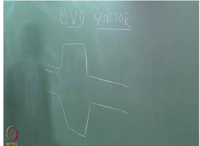
on one side of the reactor and flowing through the reactor and exiting at the other side of the reactor. There is a substrate holder or what is known as a susceptor which is fixed typically to the bottom of the reactor. It is on top of the susceptor that deposition must take place.
