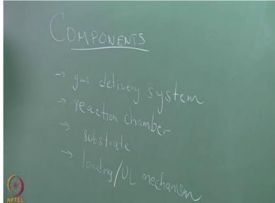
and the substrate has to be provided a separate source of energy. The reactor itself may have its own energy source so that you can maintain the entire reactor at a certain temperature and so on. But in C V D systems, typically the substrate will be maintained at a temperature that is different from the reactor itself.
