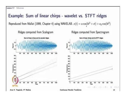
Let us look at an example where the wavelet ridges really perform a poor job and the STFT ridges perform a very good job. That is a case for the sum of linear chirps again borrowed from Mallat's book in chapter 4, and expression for the some of linear chirps is given on the top, the ridges computed from scalogram are shown on the left, and the one computed from the spectrogram are shown to the right. It is clear from this plot here that
