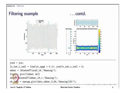
So, here is the result of that. The mat lab code for doing this is given below. What I am doing here is in the second row, line of this code and finding out the time and frequency indices of those values of the spectrogram that are less than 0.1 in magnitude. Of course, you can ask what is the sanctity about the point from. There is nothing, no sanctity about it.
