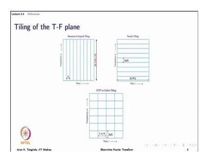
Now, what I would like to do is, with the help of this time frequency tiling idea that is commonly used, reinforce a concept of short time fourier transform in the context of time frequency analysis. Now, let me explain these 3 figures to you which will help you understand what short time fourier transforms do. And, later on, we will use this tiling again to illustrate the idea or the concept of discrete wavelet transforms, or in general wavelet transforms.
