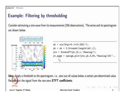
The next topic in the agenda for this lecture is to show you how you could use short time fourier transform for filtering. You have already seen how you can use the spectrogram for time frequency analysis where you plot the energy density in a 2 dimensional plane, search for features, oscillatory features or other features of interest, and then extract those features.
