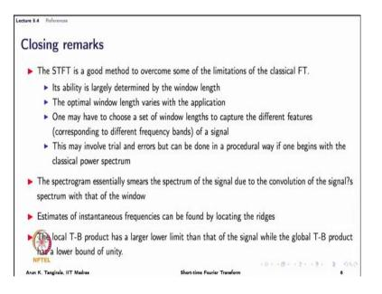
So, this is the summary of what we have learnt until now. I just want to highlight main points. One - that the short time fourier transform is definitely a significant improvement over the fourier transform in getting the time localization, but it is largely dependent on the window properties such as window length and window type; mostly window length governs the ability of the short time fourier transform to get the time frequency local features for you.
