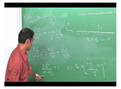
So we have the same equation which is given earlier. It was dou vx/dou t, okay. This was the governing equation that we had initially, the transient term being balanced by the viscous term. So right now this was a dimensional equation. We used those scales which were given there to nondimensionalize this particular equation. So we get rho\*U0 here\*dou V star/dou t star. So the timescale was 2pi/omega.
