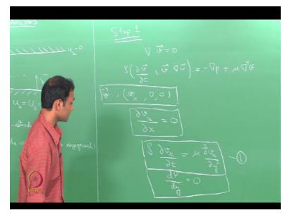
So we will go to step 1 as was discussed in the last class which is nothing but writing down the governing equations in the dimensional form. So as in any fluid flow problem, the continuity equation and the Navier-Stokes equation are the governing equations. So we have the 2 equations given as these, okay. So we have the continuity equation which is nothing but mass conservation and we have the Navier-Stokes equation which is nothing but Newton second law right for the fluid, okay.
