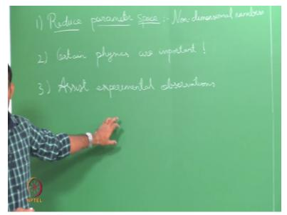
Scaling is important because first it helps to reduce the parameter space. So, by this what I mean is that if you see any fluid mechanic problem, obviously the flow field would depend on the viscosity, density and other pressure that is applied, the length scales near the channel, how large the diameter of the pipe is and things like that. So, what scaling helps us is to reduce the parameters that are affecting the flow. So, you can club all the parameters to essentially lesser
