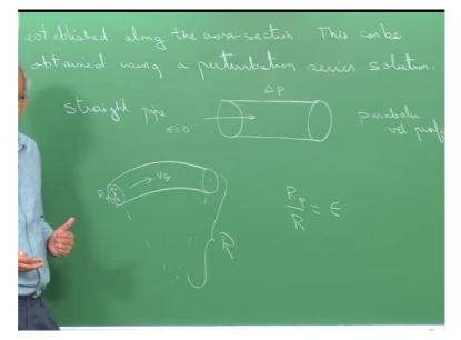
There are vortices or circulation patterns established along the cross section. So what we wanted to do is we wanted to find out this flow field where the velocity field gets modified. In the straight channel, you have only the axial component of velocity, you do not have any other component v theta okay.
