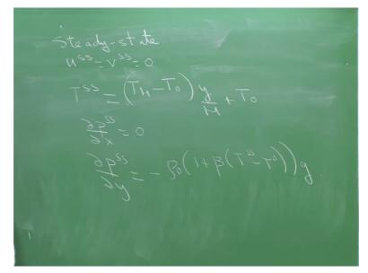
Steady state is uss=vss=0, Tss is TH-T0 times y/H+T0 and dpss/dx is 0, dpss/dy=-rho0 times 1+beta times Tss-T0 times g and that is the steady state whose stability we will be finding out in the next class. Thank you.
