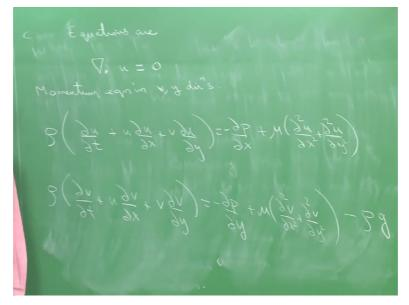
Equations are the continuity equation, which is divergence of u=0 okay and says I am neglecting things in the z direction, I do not write the momentum equation in the z direction. I am just going to write the equation in the x and y direction okay. Momentum equation in the x and y directions what is that? This is in the x direction right. So this is x direction and the gravity is not in the x direction and then I have this.
