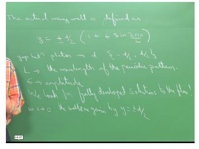
So the actual wavy wall is defined as y=+d/2 is the top surface the bottom surface will be -d/2 then the entire channel of the thickness b okay. So epsilon basically gives you some control over what is the amplitude of the periodic nature which is imposed. So the way I am looking at this problem that is a constant value d/2 so if this have been actually this is like if epsilon is 0 I reduces to the problem of flow between 2 flat plates which we have seen earlier. Okay.
