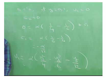
But you never know, the point I want to make here now is using the boundary conditions, what are the boundary conditions at y=0 and 1 u1 is 0, the no-slip boundary conditions okay. So this implies what? c2 is 0 and what is c1 0=alpha\*1/4-1/6+c1, which gives me c1 is alpha times 1/6-1/4, which is alpha times -alpha/12 okay. So I have got u1 as alpha times y squared/4-y cube/6-y/12 okay.
