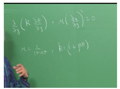
So we will continue today working on the problem of incorporating the effect of viscous heating in a viscometer okay and one of the thing we are going to see is that the estimation of the viscosity, if you neglect viscous heating what is it going to be and when include the effect of viscous heating how is it going to be effected? So that is the whole idea because viscosity is the function of temperature okay.
