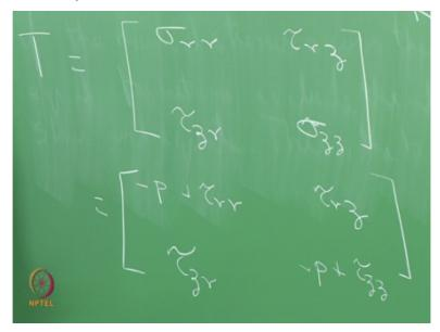
I am going to make sure, I do not make this mistake I made last time, sigma rr tau rz tau zr and sigma zz, okay. Just to tell you that in the normal direction, we are using sigma to represent the total component and now I am going to break this have been in terms of the pressure and that due to the flow, okay. So, now I am going to write this as -P + tau rr and this is what I sure, I have done last time -P + tau zz, okay.
