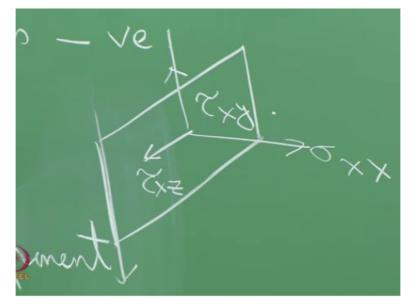
Now, what are the other components which are acting on this surface? Other components acting on this surface include tau x, y because my surface is fixed okay, it is a tau x, y and this is the stress component in the y direction but is acting on the surface x + delta x and tau x, z is the stress component in the z direction. So, the way I have drawn this tau x, z is going to be in this direction okay and tau x, y is going to be in this direction.
