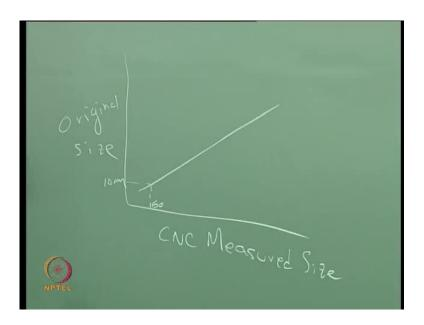
And the, and therefore, once you collect data using the condensation nuclear particle counter, you can essentially graph the original size to CNC measured size and you can show basically that there will be a correlation between them. As the CNC measured size, this will always obviously be higher than this, so, every point here, for example, the measured size may be 16 nanometers and the original size may be 10 nanometers.
