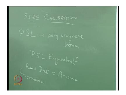
So, next well, PSL is primarily used for samples containing plastic and quasi plastic particle populations, the Arizona road dust as now emerged as a viable alternative for samples that contain predominantly metallic and silicate or alumina based constituents. So, for a something like a ceramic, you are more likely to use the road dust as your calibration standard.
