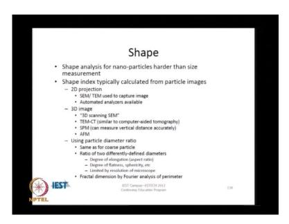
Now, switching over to shape analysis, shape is a qualitative measure, unlike size, which is qualitative. And therefore, shape analysis is always harder compared to size analysis. Now, shape just like size, can be obtained through projections. So, you can take a three-dimensional object projected onto three-dimensions or a 2D plane and obtain shape that
