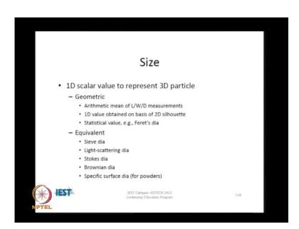
Now in terms of size analysis, we have seen several methods in this course earlier. Essentially when we talk about size, what we are trying to do is, represent even a threedimensional particle with a dimensional scalar value. So, for example, when we represent the particle by a diameter, that is what we are doing, we are assuming that the shape of the particle is roughly spherical, and therefore, you can use essentially a single dimension to represent the size of the particle.
