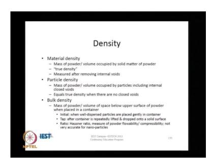
The method of density measurement, on the other hand, is something that is done in three different ways. You can assess Material density, you can assess Particle density or you can assess Bulk density.
