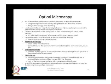
We have discussed optical microscopy earlier in our lecture, but just to recap the key points; it is a simple method, low cost, it is widely used for routine analysis, magnification less than 50 times; however, there are analytical microscopes that are available, that can provided up to 1000 x magnification. The sample is examined initially at a low magnification 5 to 7 x, and then the magnification is gradually increased, until you get a better understanding of what you are looking at.
