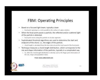
Now, the beam can be any light beam, although it is a typically a laser. And here again, you try to train the focal point on the particle, and when the focal point of the light meets the particle, you measure the reflective light and/ or the scattered light.
