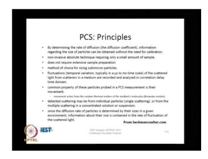
Now, Photon Correlation Spectroscopy is actually only another name for DLS, the Dynamic Laser Diffraction based methodology. Here, what we are really doing is determining the rate of diffusion or the diffusion coefficient of the particles.
