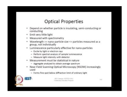
Optical properties, as we have seen, they certainly change with particle size. The optical behavior of nano-particles will depend on whether it is an insulating particles, semi conducting or conducting particles. Nano-particles on their own do not emit light very much, again light emission is a surface area dependent property, so as particles become smaller, the emission of light decreases just as scattering decreases.
