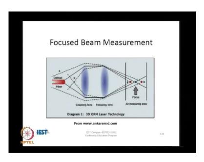
The Focused Beam Measurement technique is one that, again similar to light scattering, in the sense that, you take an energy beam and you focus it on the particle.
