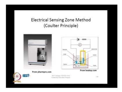
The Electrical Sensing Zone Method, also known as the Coulter Principle, is a little different from the techniques we have discussed so far, in the sense that, here the particles are actually immersed into an electrolyte solution and the change in conductivity is measure. So, this is particularly well suited to non-conducting particles.
