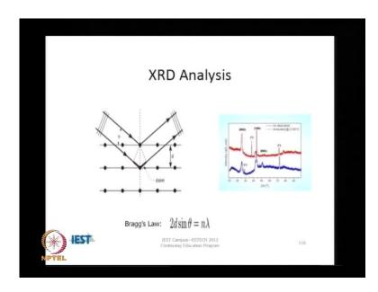
XRD, again we have discussed in some detail in class, it is the primary method that is used to detect the crystallographic structure of a material, and it operates by the principle of Bragg's law, which can enables us to measure inter planar distances in a crystalline structure, by looking at scattering intensity.
