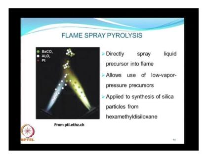
Flame spray paralysis is a combination of two methods that we have discussed earlier, flame pyrolisis and spray pyrolisis. Here, thus the liquid is sprayed directly into the flame, so the liquid precursors are injected into the flame.
