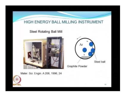
However, more recently they have been advances in ball milling technology, in particular, the high energy ball mill which is an improvement over the conventional ball
