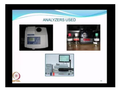
Sound the analyzers that are used for testing particle compositions and sizes and counts are shown here. The left hand side top picture shows at turbidity meter, you may recall that we discuss this in the context of measuring particle concentrations in suspensions, turbidities are measure of the total scattering intensity of particles in suspension. So, it can be used as a qualitative measure of particle size as well as particle concentration in liquids.
